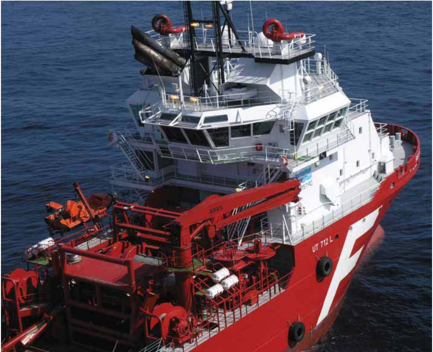
The Far Sound UT712L built in 2007. This is a medium sized anchor-handler with all possible accessories, and its 16,000 bhp shows that the way forward may not always be to build bigger. Picture: Victor Gibson
