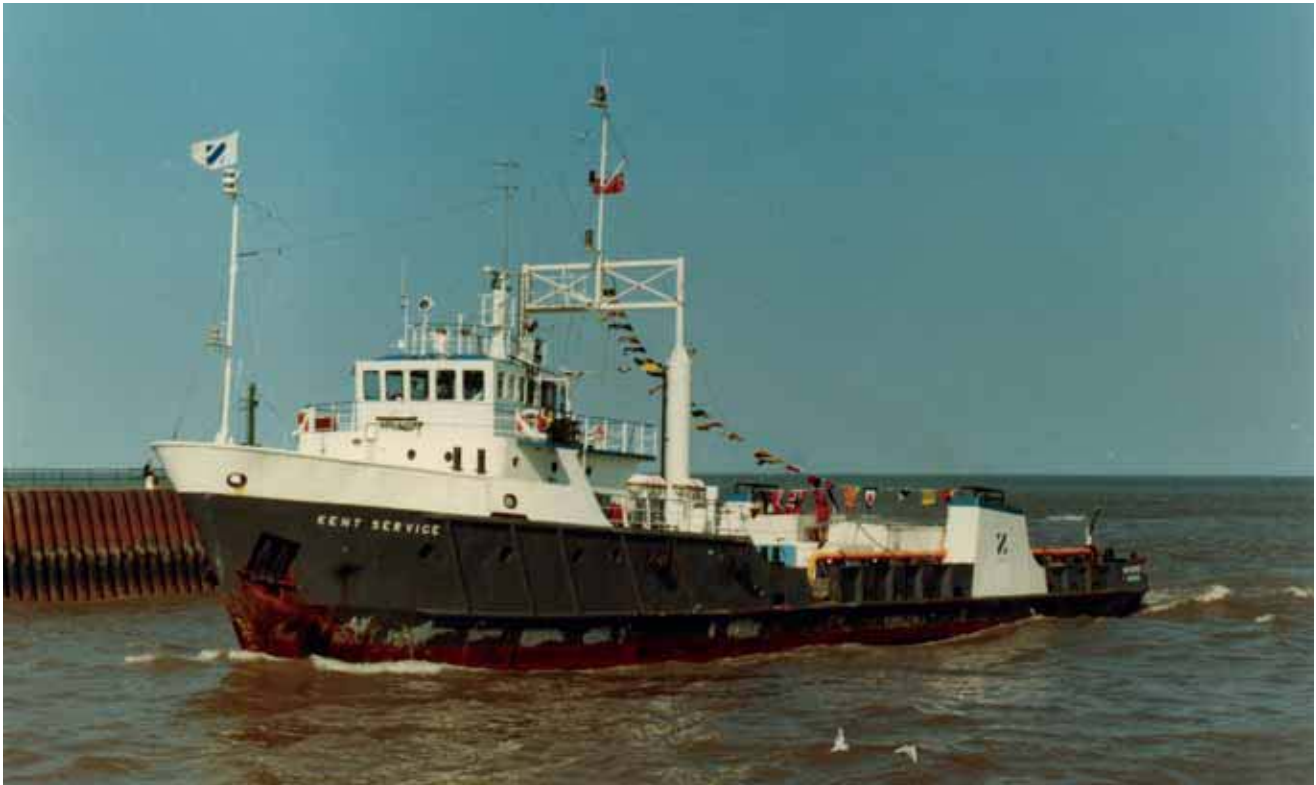
This ship was originally the Kent Shore built in 1967 for Offshore Marine, one of a number of sister ships powered by Lister Blackstone engines developing 1600 bhp. Picture: Paul Gowen
