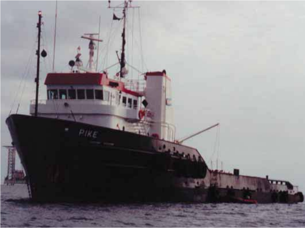
The Pike a 1980s built Halter Marine 180 footer, a ship type still used in many places of the world for moving jack-ups. Picture: Fergus Mack.
