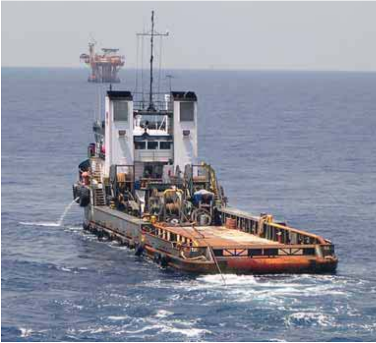
The Hatch Tide. Built in 1982 at Halter Lockport. The enlarged funnels alone cannot hide the lines of the standard Halter Marine design. The towing gate is still in use. Picture: Ron Jansen.
