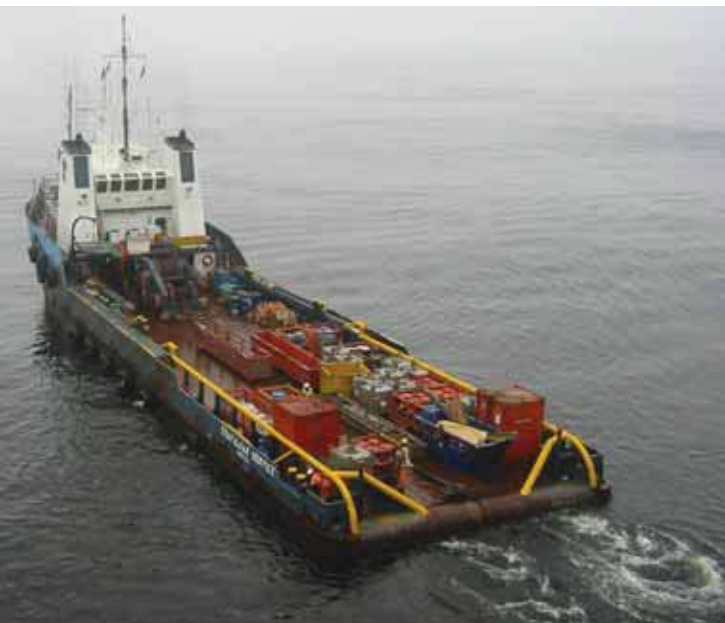
The Trafalgar Service. Built in 1983 by Halter Marine. The engine exhausts still rise out of the afterdeck and are plumbed forward to the "North Sea Stacks". Photo: Sandy Stewart.
